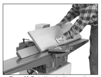
Figure 26. Typical bevel cutting operation.
